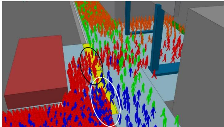
**Figure 2.** MassMotion Simulation During Egress at Gate One and North Walkway (Channel One: white circle, Channel Two: black circle)
