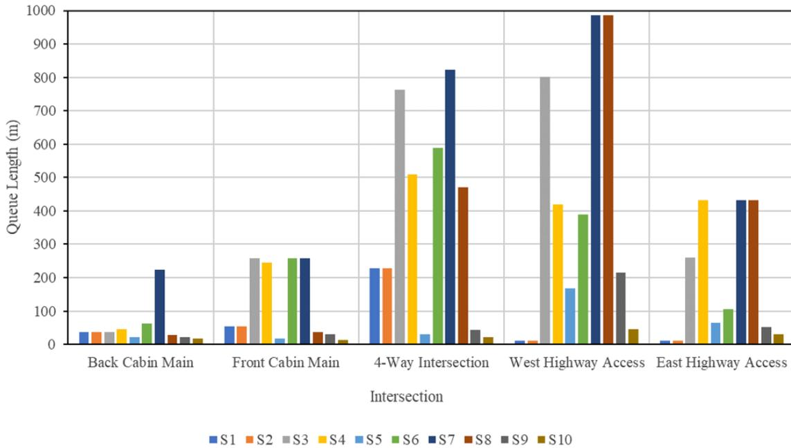
Fig. 9. Maximum queue lengths for main network intersections
