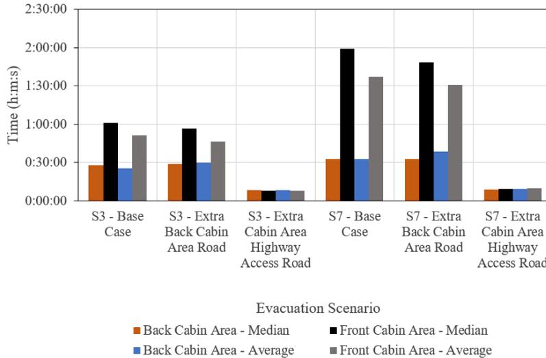
Fig. 7. Aggregate average and median individual evacuation times for the worst-case scenarios with additional egress roads
