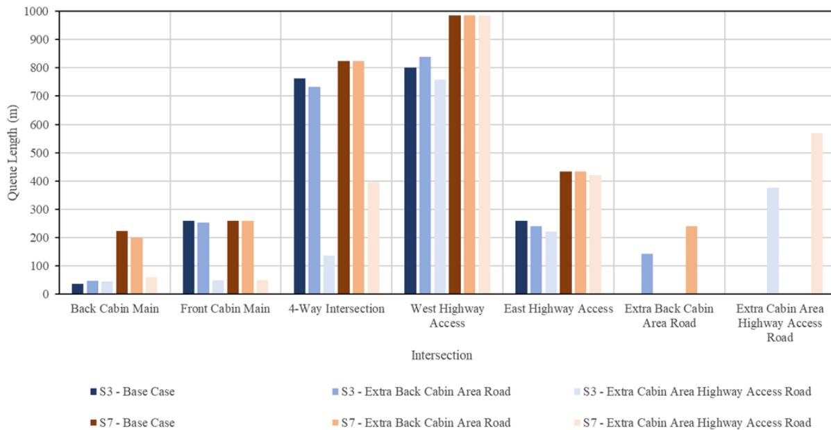
Fig. 10. Maximum queue lengths for main network intersections on the worst-case scenarios with additional egress roads
