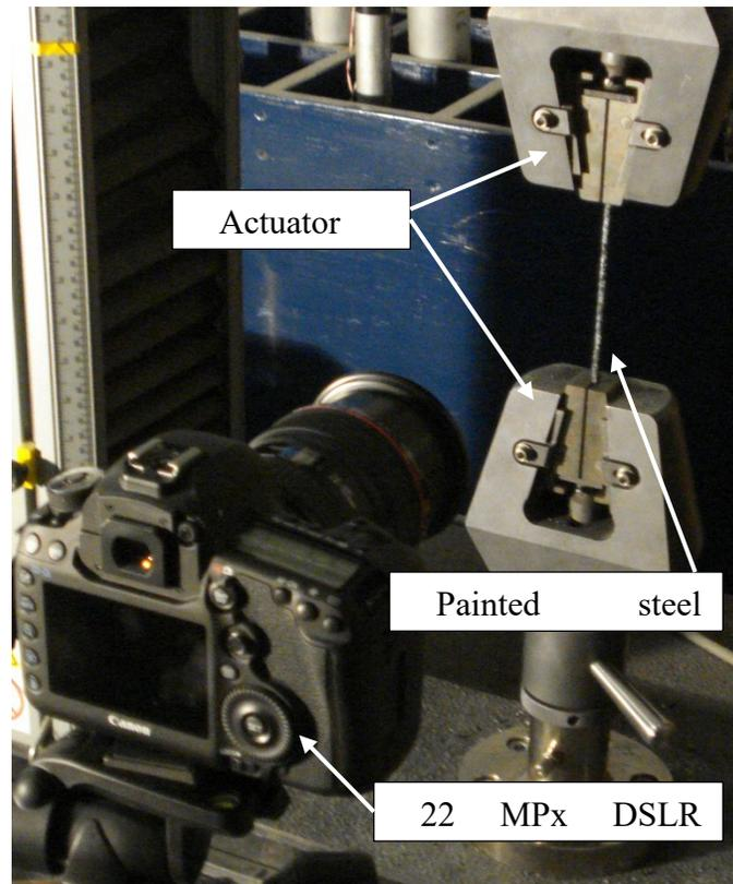
**Figure 1.** Loading apparatus with digital image correlation.
