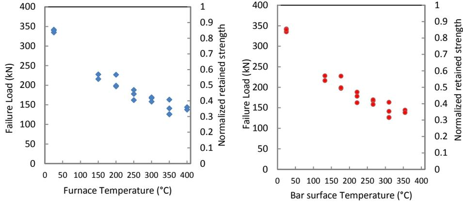
**Figure 4. Tensile strength degradation in steady state tests (#5 GFRP bars): (Left) as a function of furnace temperature; (Right) as a function of bar surface temperature**
