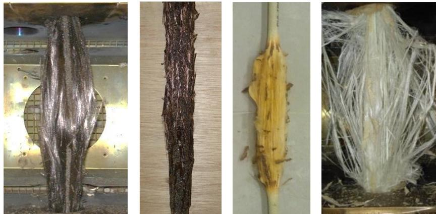
**Figure 6. Samples after transient test: from left to right applied tensile loads are 75, 120, 160, and 200 kN, and failure temperatures are 547, 450, 340 and 160 °C respectively**
