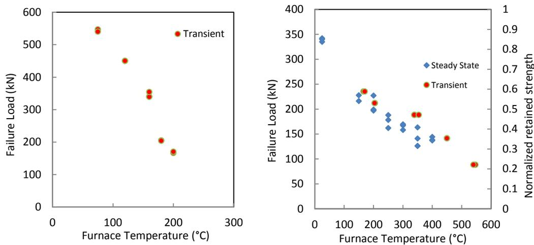
**Figure 5. (Left) Tensile strength degradation in Transient tests (#5 GFRP bars); (Right) comparison of transient test results to steady state tests**
