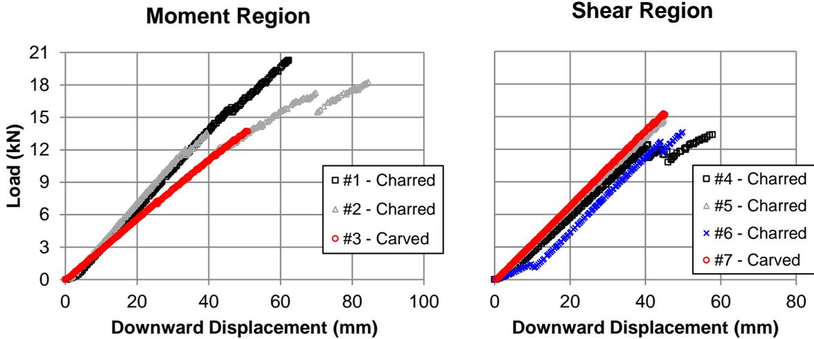
Figure 5: Load versus downward displacement of the carved and charred beams that have been damaged in the moment region (left) and shear region (right)
