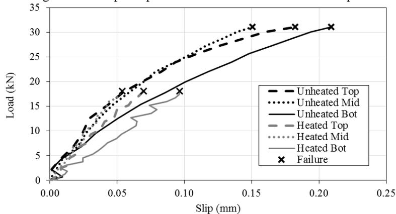
The trends show that the heated samples follow similar trends to the unheated samples, however they exhibit a more brittle adhesive failure. This could be due to adhesive damage from the elevated temperatures as resins cannot typically be melted and reformed like some other polymers, but rather they degrade. This behavior could explain the reduction in residual shear stress seen in Figure 7.
