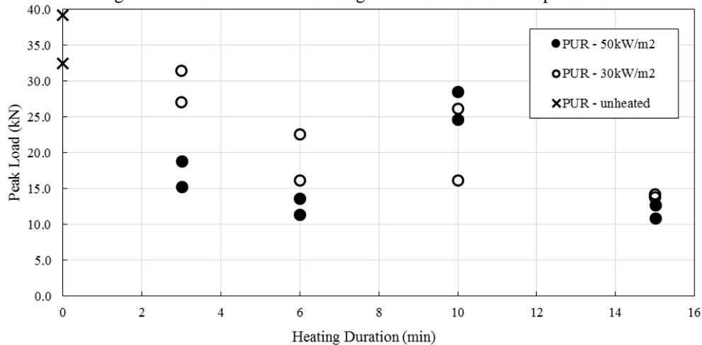
Figure 6: Peak loads versus heating duration for PRF test specimens
