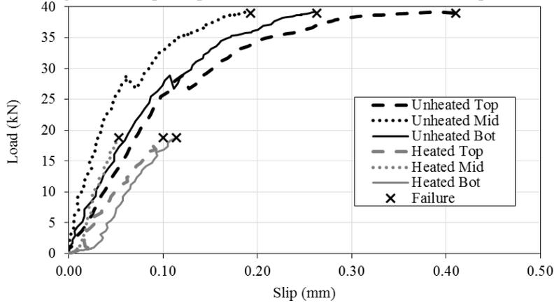
Figure 10: Sample slip versus load trends for two PRF samples
