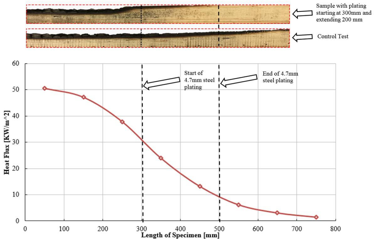
Figure 7: LIFT Testing and Imaging Technique Result
