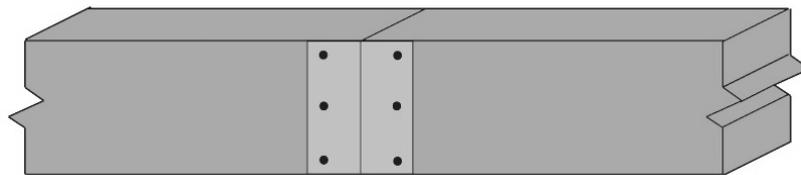
In this sense, the pyrolysis and charring of the LVL under the steel plates is also studied herein. The char depth was measured using the same process as the control heat flux and the samples were cut down the centerline to measure the depth, as per the standard ASTM 2013 E1321<sup>5</sup>. These tests are underway at the time of publication.
