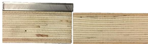
The LVL for these samples was obtained from a manufacturer in Ottawa, Ontario. The adhesive used in this LVL is proprietary to the company. This is quite common with EWP products. A series of 44.5mm by 240.0mm Grade 2.0E single ply LVL beams were acquired and cut down to 100mm x 100mm x 44.5mm test samples. The samples have a coating on the exterior faces for weathering, which is green in colour, and this coating was left on for the testing. See Table 1 for test schedule.
