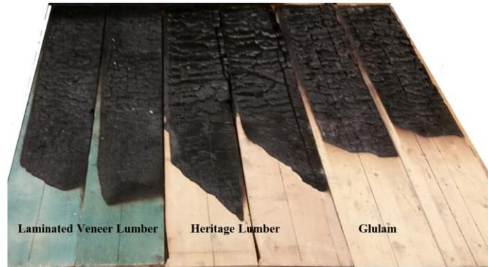
Figure 10. Timber Specimens after Heating.
