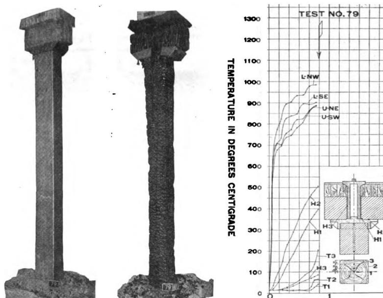
Figure 6. Early Standard fire tests were conducted on timber columns in the early 20<sup>th</sup> Century. It was difficult to control these tests due to the heat given off from the timber. Excerpted are the results of the first Standard fire test on un-encapsulated timber (Ingberg 1921).
