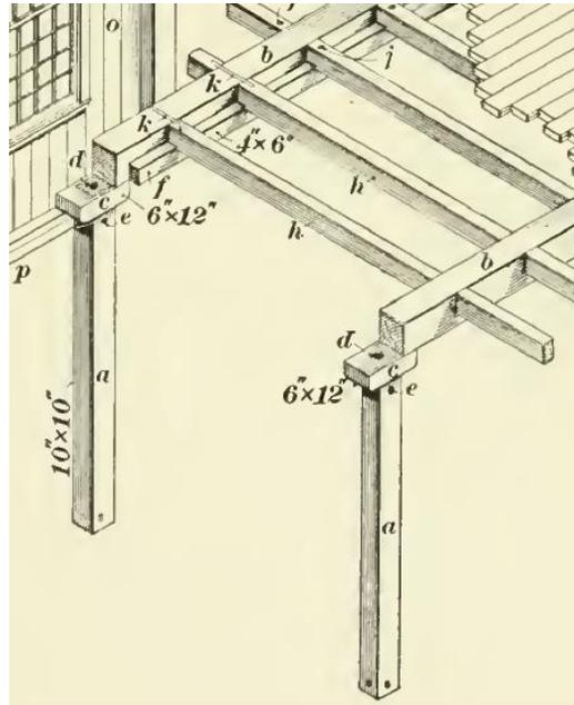
Figure 2. Solid timber was prevalent for a 19<sup>th</sup> century industry structure design called slow-burning construction (see Scanton 1899). The timber would be made sufficiently large so that business continuity was ensured if fire damage occurred. The timber would have a hollowed center, which would aid in connection and prevent moisture accumulation that would enable rot.
