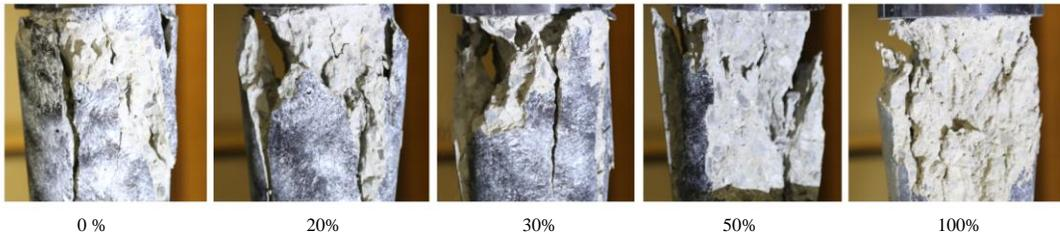
Figure 8: Failure planes with various recycled cement substitution
