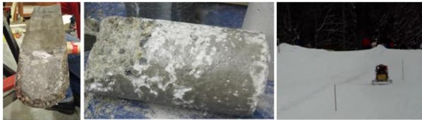
Figure 9. In an experiential learning exercise students utilized the RCC replacing 20% of the ordinary cement to meet green and sustainability objectives in the concrete toboggan competition in Canada.
