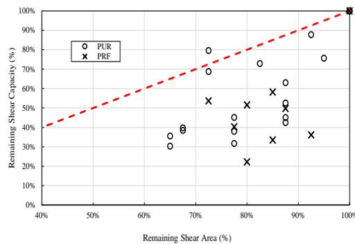
Figure 7. Adhesive breakdown after fire exposure (Quiquero and Gales, 2017)
