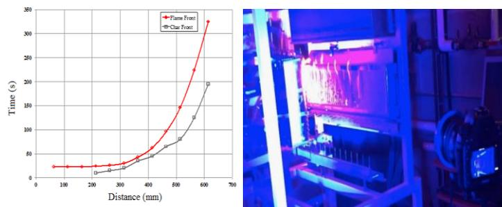
Figure 9. Measured Flame spread versus Char formation of Solid Timber using Selective Filtration
