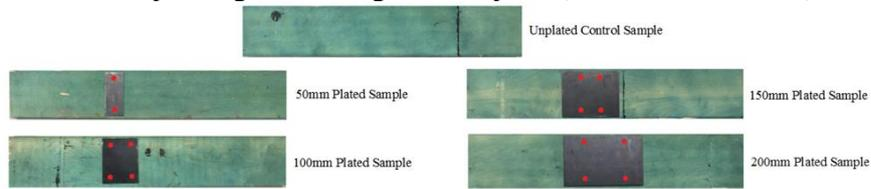
Figure 12. Flame spread connection tests
