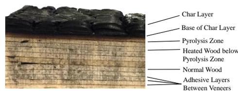
Figure 3. Timber breakdown (Laminated Veneer Lumber shown)
