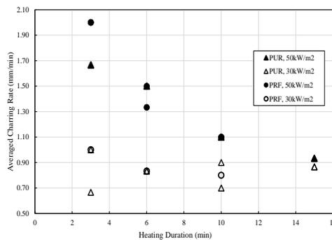
Figure 6. Charring behavior versus exposure time (Quiquero and Gales, 2017)
