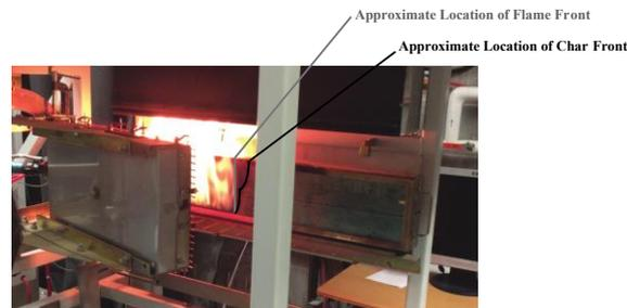
Figure 8. Pyrolysis Mechanisms for exposed timber
