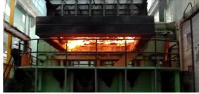
Figure 11. CLT Standard fire floor test conducted in 2014 (authors' photo; see Su et al., 2014).
