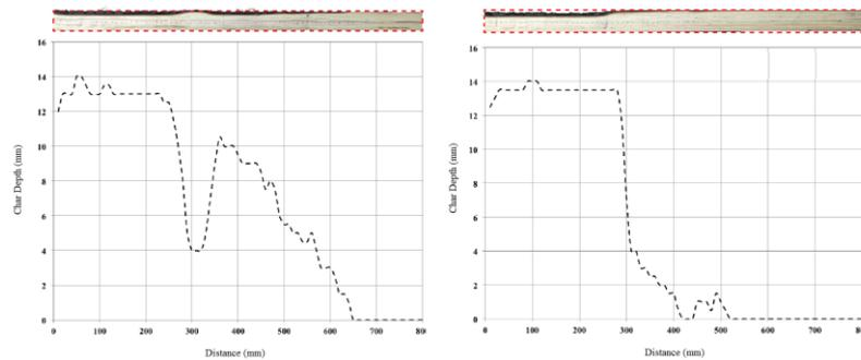
Figure 13. Char depth results of flame spread connection tests (50mm plate, right 200mm plate).
