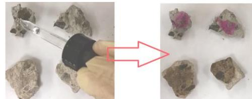
Fig. 2. A carbonation test is performed with the students to illustrate material chemistry.
