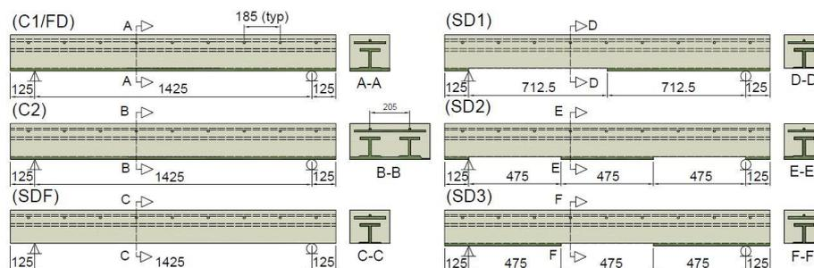
Fig. 1. Control and simulated damage specimens
