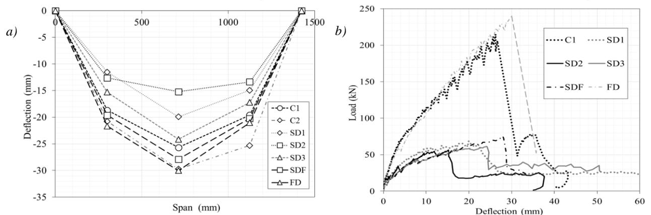
Fig. 4. a) Span-deflection at ultimate; b) Load-deflection responses of damaged strips
