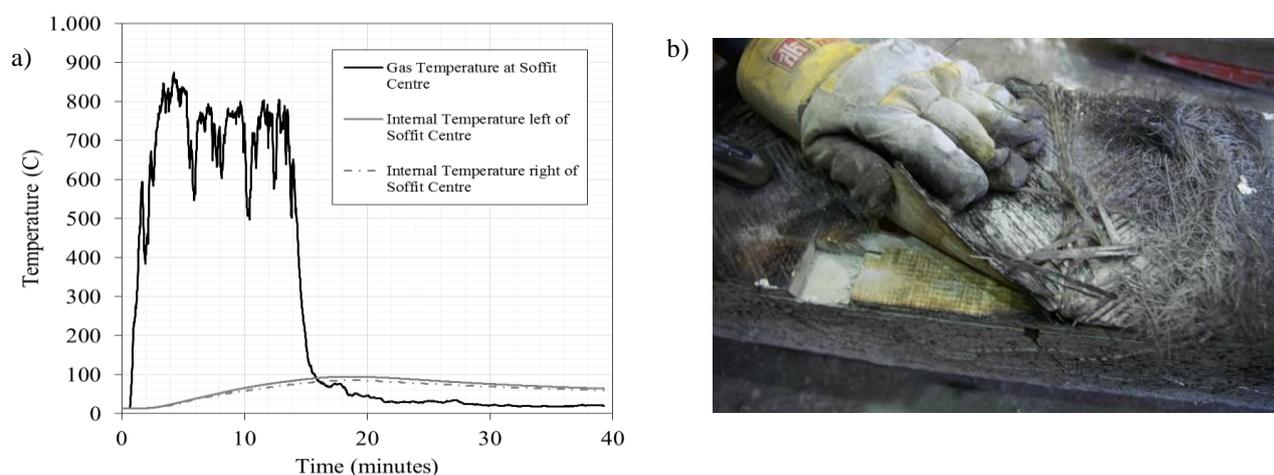
Fig. 7. a) Time-temperature history for Specimen FD; b) Delaminated pyrolysis/char layer on GFRP base plate
