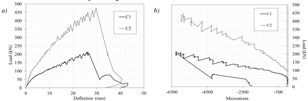
Fig 3. Control specimen strain responses: a) Load-midspan deflection; b) Midspan compressive strain
