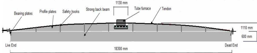
**Figure 1: Strongback frame and custom tube furnace configuration.**
